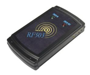
The RF503 is ideally suited for IN/OUT tracking of personnel at seminars, conventions or other temporary installations. With its built-in memory and clock it independently reads, timestamps and logs every transaction. The transaction is clearly and automatically indicated as IN or OUT each time a user presents their badge. These transactions can be downloaded at a later time to determine the duration and times each user was on premise.
